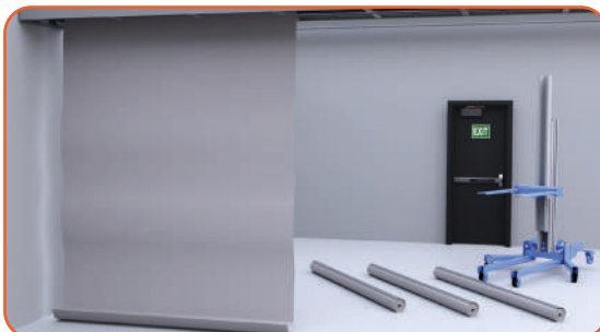
Slide the wall panel to 3" from the wall
