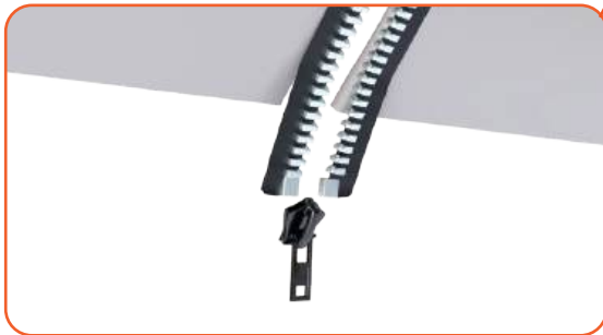
Start zipping from the bottom Note: Make sure both walls are aligned
