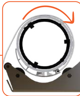
Rotate the tube facing down and insert the screws
