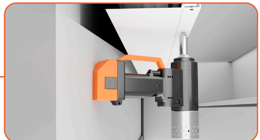
Use Rivet Gun to connect the housing cover
