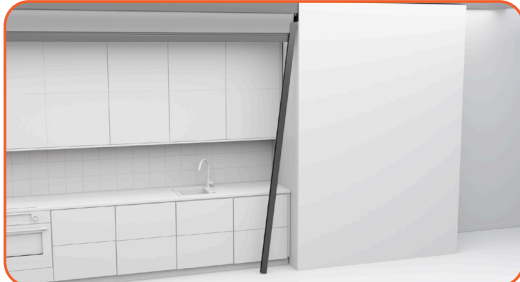
Lift side guides against either side of wall
