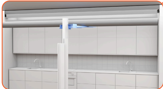
Use material lift to raise large panel to small panel (zipper facing up)
