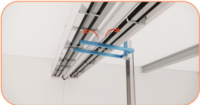
Lift the tubes to the center of housing
