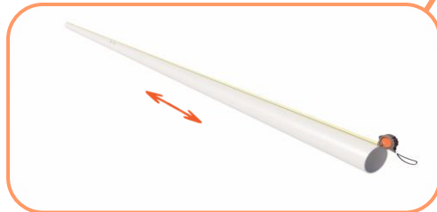
Measure the length of the tube based on the wall's measurement and prepare to cut out the excess and 3"
