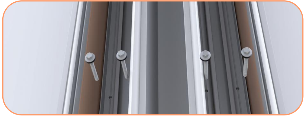
Insert the bolts into the side guide
