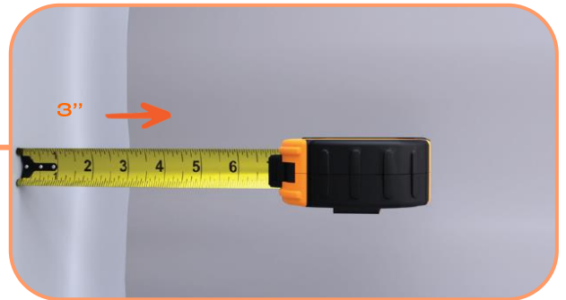
Measure a 3" setback both sides of the wall
