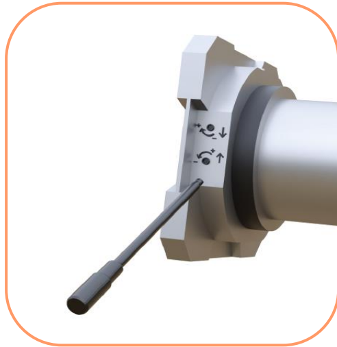
Ensure that the limit adjusters are on the bottom of the housing (facing the floor)
